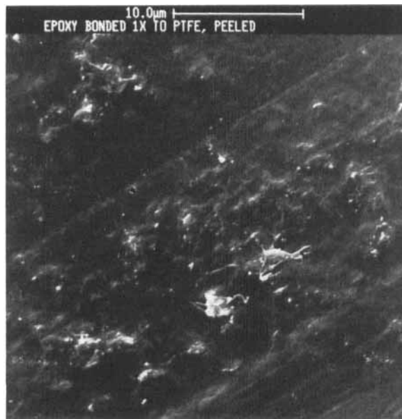
FIGURE 7 A scanning electron micrograph of the epoxy side of an adhesive joint to PTFE that had been bonded once.
