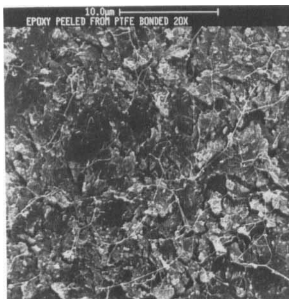
FIGURE 10 A scanning electron micrograph of the epoxy side of an adhesive joint to PTFE that had been bonded twenty times.
